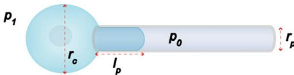
**Fig. 5** Schematic diagram of micropipette aspiration. In this setup, the cell is suspended in fluid of pressure  $p_1$  and a micropipette of radius  $r_p$  is placed on the cell membrane. The pressure inside of the pipette is then lowered to  $p_0$  and the resulting deformation of the cell membrane,  $l_p$ , into the pipette is measured. This information, along with the radius of the cell outside of the pipette ( $r_c$ ), can be used to determine the cell’s tensile modulus and viscosity
