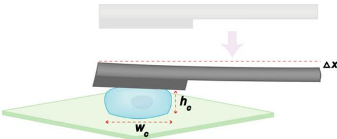
**Fig. 1** Schematic diagram of the cytocompressor. To test single cells under unconfined compression, the cytocompressor uses a cantilever beam with a wide probe attached to its end. A piezoelectric actuator precisely moves the cantilever probe assembly toward the cell surface, and compresses the cell a set amount. Compression events are recorded via a CCD camera, and cell height ( $h_c$ ) and width ( $w_c$ ) are determined from extracted frames
