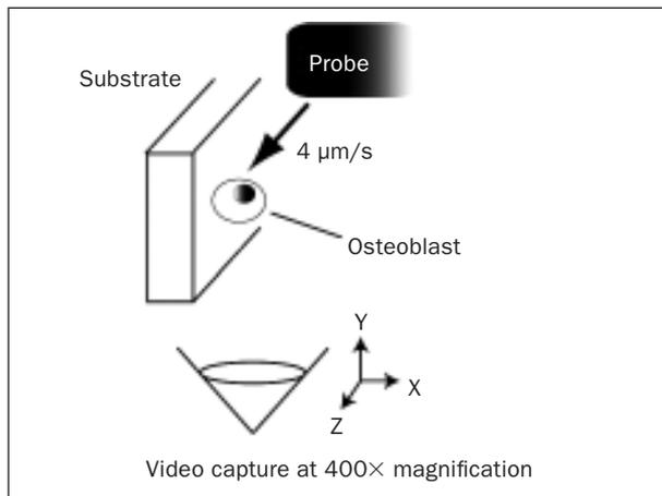
**Fig 1** Diagram of the cytodetachment machine.
