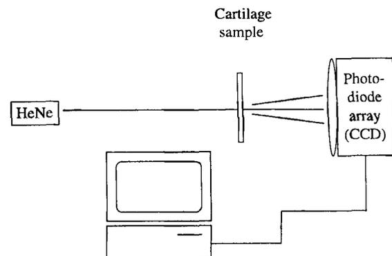
FIG. 2. Experimental setup. CCD = digital camera.
