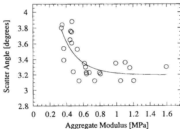
FIG. 3. Plot of average scatter angle, as defined by Eq. 1, relative to aggregate compressive modulus. The solid line represents the theoretical result, Eq. 8, using values for the fit parameters given in the text.
