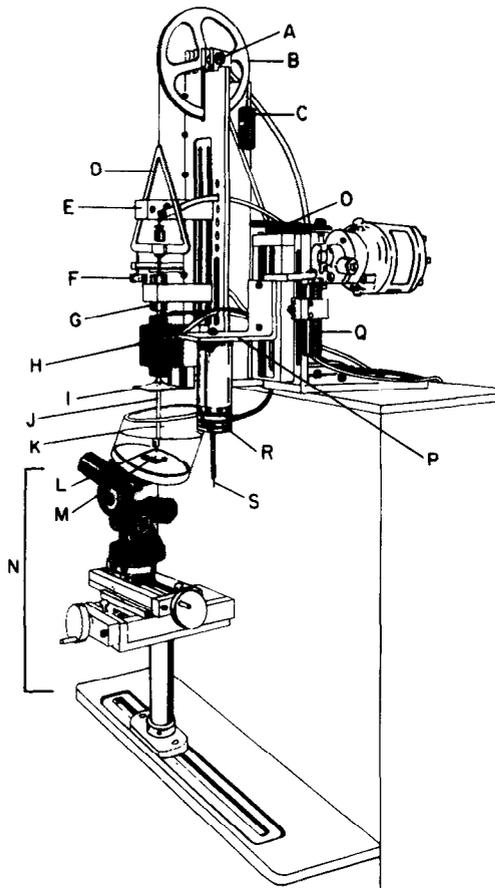
Fig. 3. The biphasic indentation apparatus featuring a porous-permeable indenter tip (L), a six degrees of freedom specimen mounting frame (N) and a thickness measurement probe (S). See text for design and operational details.
