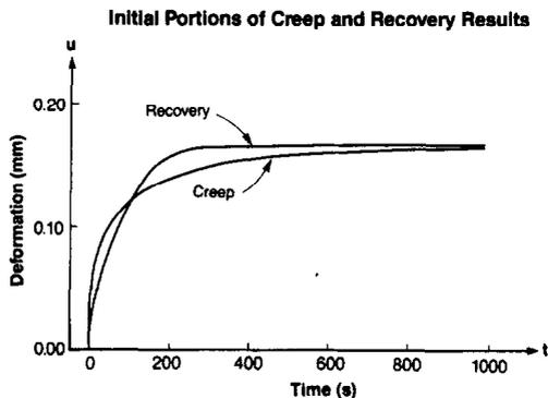
Fig. 4. Comparison of the rate of creep and the rate of recovery in a typical biphasic indentation experiment.
