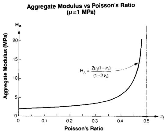
Fig. 6. Theoretical relationship between the aggregate modulus ( $H_A$ ) and Poisson's ratio ( $\nu_s$ ) of the solid matrix for  $\mu_s = 1$  MPa.
