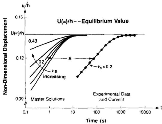
Fig. 2. Schematic depiction of the time-shift method where a master solution is shifted by an amount  $S$  along the  $\log_{10}(t)$  axis. Diagram illustrates how the 'shape' of the displacement curve is controlled by the parameter  $\nu_s$ , for a given set of  $P_0, u(\infty), a/h$ .
