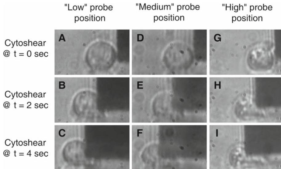
**Fig. 3** Alterations in cellular morphology and position of chondrocytes experiencing direct shear. The entire mechanical event is video recorded and subsequently analyzed to yield mechanical properties and indicators for cell movement. Differences can be observed when the probe is placed in its low position (a–c), medium position (d–f), and high position (g–i) during the time course of shear application. Most
