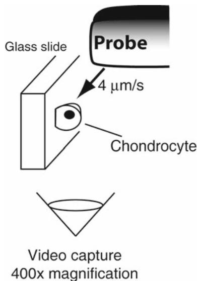
**Fig. 1** Illustration of the experimental setup for studying single cells experiencing direct shear. A piezoelectric actuator drives a shearing probe laterally toward an articular chondrocyte seeded onto glass slides. Through visualization on an inverted microscope, the probe height can be controlled during the experiment. The entire mechanical event is further recorded through a CCD video camera connected to the microscope. The figure is not drawn to scale
