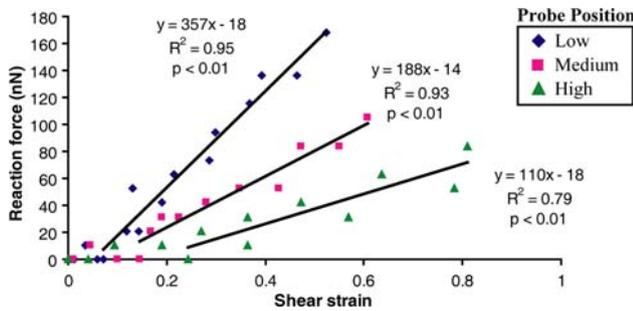
**Fig. 4** Representative force plots of single chondrocytes experiencing shear from different probe heights. Force values are typically minimal until around 15–20% applied strain, after which a significant increase in force is observed. In addition, the slope of force versus shear strain is noticeably different among the three probe heights, with the low probe height generally inducing the greatest slope in force accumulation
