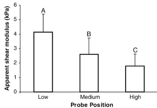
**Fig. 5** Apparent shear moduli as a function of probe height. Single chondrocytes are perceived to be stiffer when the probe is placed lower to their base, with significant differences ( $p < 0.05$ ) observed among all three groups. This suggests that the cell is non-uniform in its mechanical properties along its vertical axis. Data presented as mean  $\pm$  standard deviations
