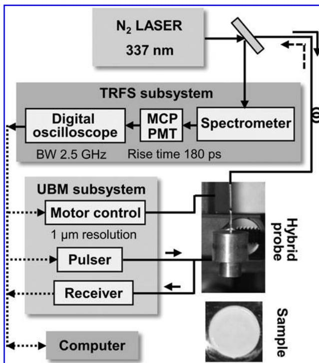
**FIG. 1.** A schematic diagram of the combined TRFS-UBM system including laser source module, TRFS subsystem, UBM subsystem, and the combined probe (transducer and fiberoptic). A tissue engineered cartilage sample (at  $t = \text{week } 4$ ) is shown. TRFS, time-resolved fluorescence spectroscopy; UBM, ultrasound backscatter microscopy; MCP, multichannel plate; PMT, photomultiplier tube.
