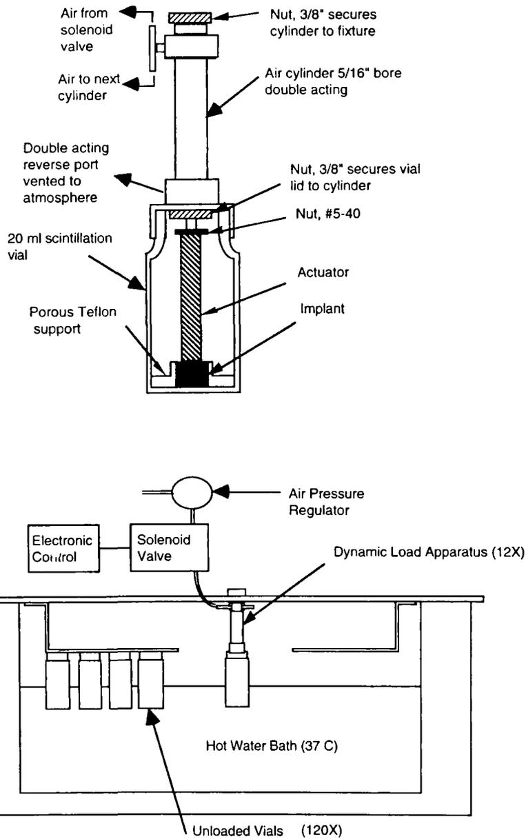
**FIG. 1.** Dynamic loading fixture. The dynamically loaded implants were rotated through the 12 dynamic loading apparatus for 90 min each day. The air cylinder applies an area equivalent constant force load of  $1 \times$  body weight every 2 sec. A pressure regulator precisely controls the air pressure to the cylinder, resulting in a constant force load imparted on the implant. Control implants degraded under nonloaded conditions.
