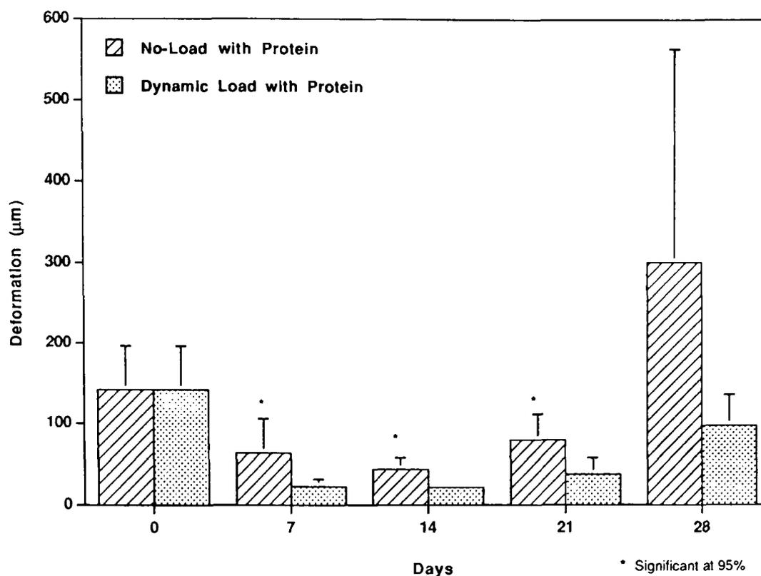
**FIG. 5.** Implant surface deformation. Compared with the nonloaded condition at each sample time point ( $p < 0.05$ ), dynamic loading significantly stiffens the implants ( $p < 0.05$ ), with a maximum stiffness at the end of the second week. Results shown as mean  $\pm$ SD.
