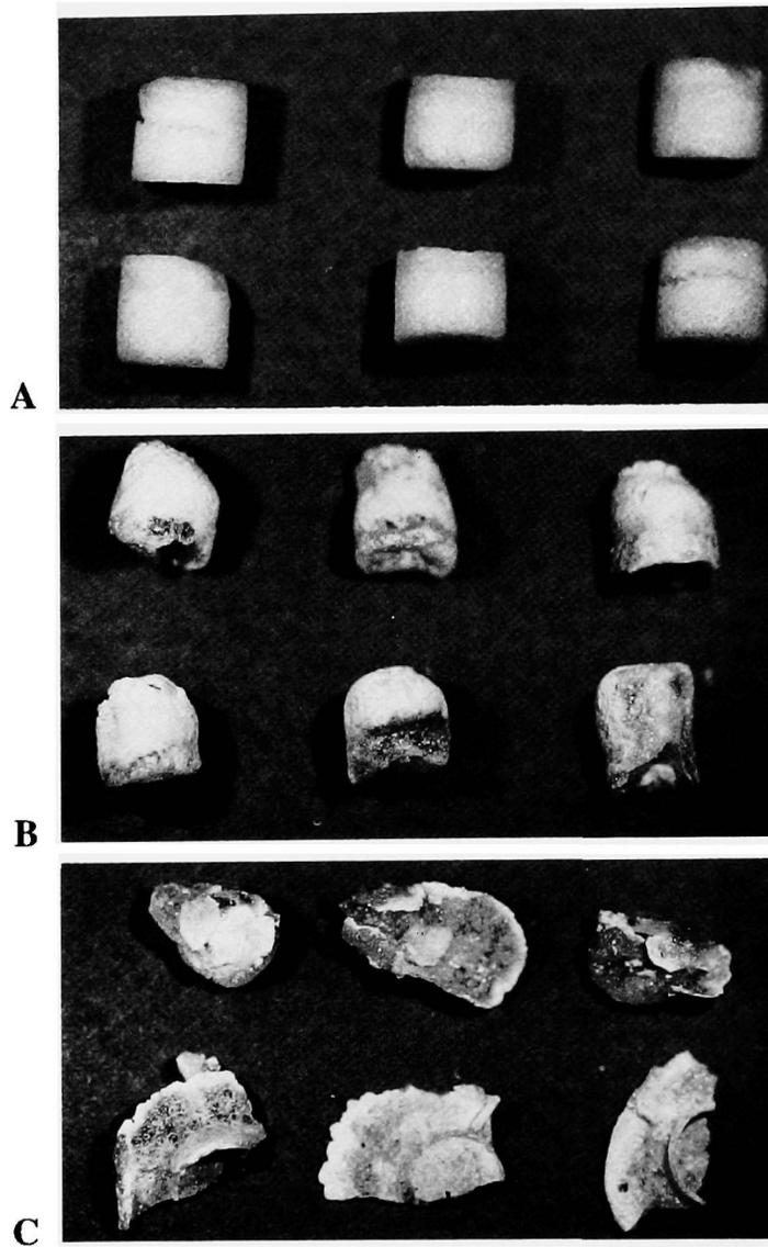
**FIG. 6.** Implant gross morphological changes. Specimens shown have been freeze-dried and photographed at  $2.5\times$  magnification. (A) Day 0, (B) day 42 of nonloaded degradation, (C) day 42 of degradation of dynamically loaded implants. Dynamic loading significantly deforms the implants by the end of the sixth week.
